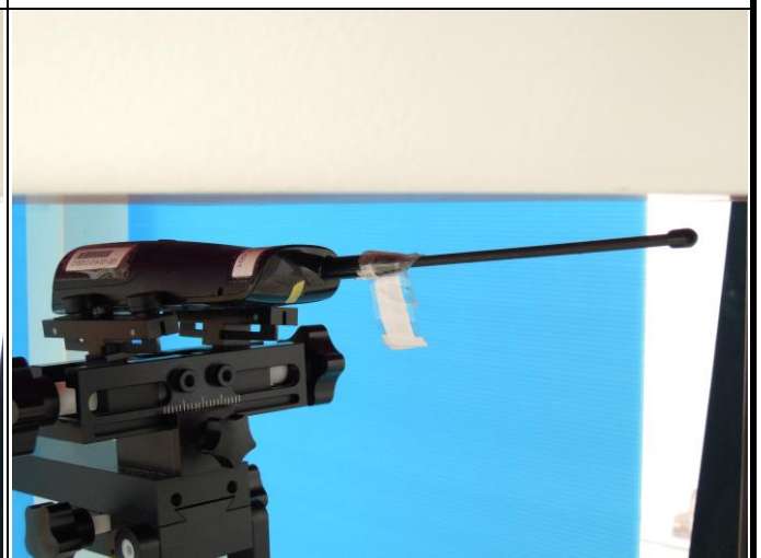
Phone + Ant-1 – Rear Face with 1.5 cm Gap
