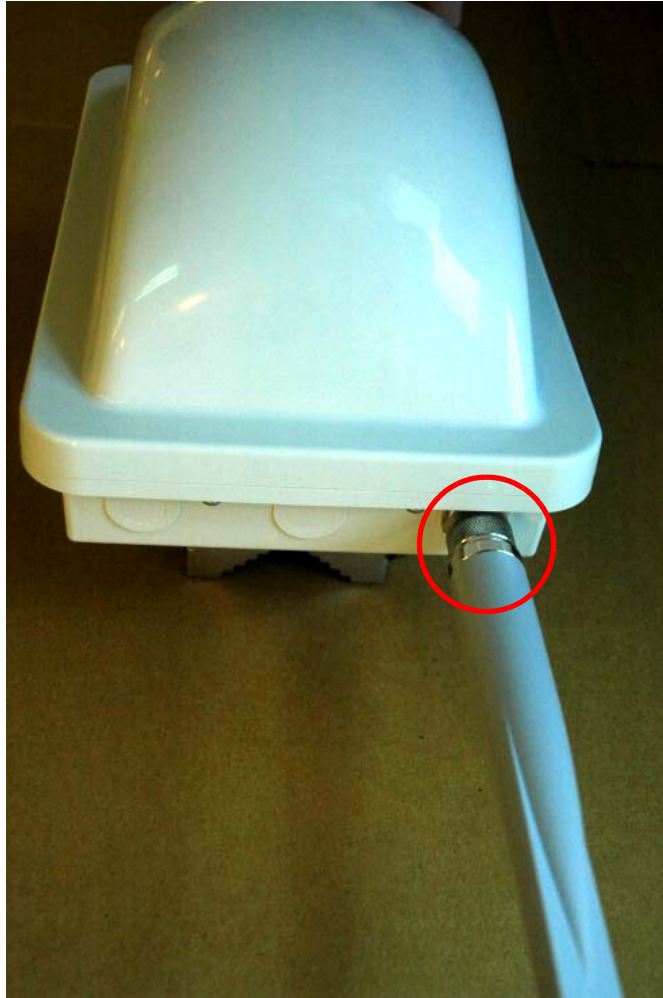
Figure 33. Connect the standard N-type male connector to the standard N-type female connector on the Access Point
