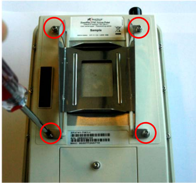
Figure 19. Tighten the four machine screws to fasten the bracket to the Access Point
