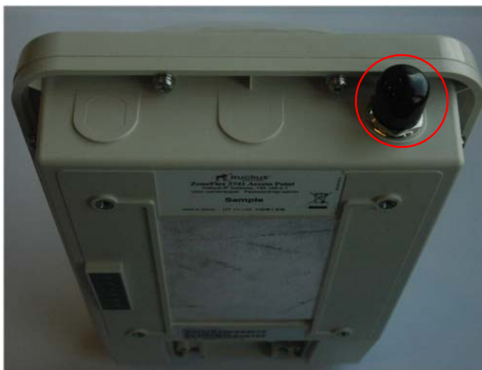
Figure 2. The antenna connector is protected by a black waterproof antenna connector cover
