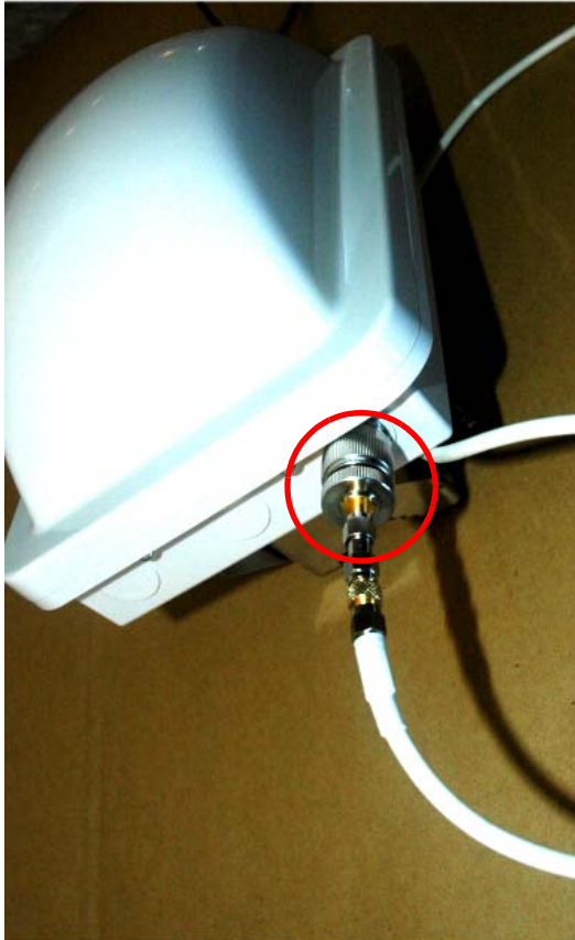
Figure 32. Connect the RF coaxial cable to the standard N-type female connector on the Access Point.
