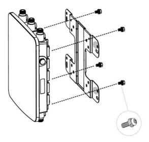
4. Tighten the flat washers to secure the bracket to the mounting surface.
