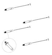
3. Place the lock and flat washers on the four hex cap screws and drive the screws to attach the bracket to the back of the OAP725AG.
