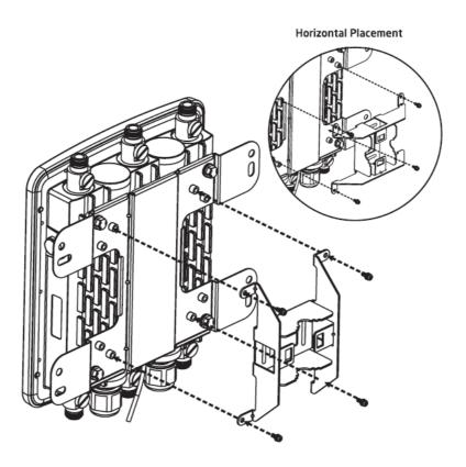
3. Thread the open end of the Pole Strap through the two tabs on the Pole Mount Bracket.
