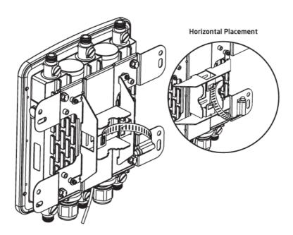
4. Lock and tighten Pole Strap to secure Pole Mount Bracket to the Pole.
