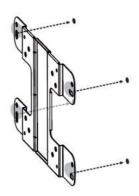
2. Drill a 37mm deep 8mm hole in the markings and hammer the bolts into the openings.
