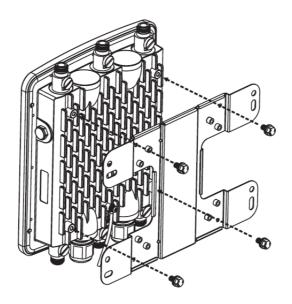
2. Drive the four round head screws to attach the Pole Mount Bracket to the bracket.
