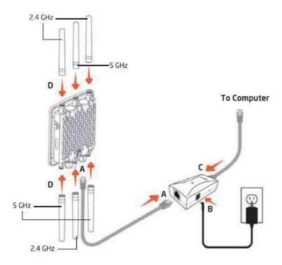
**Note**: The OAP7250AG can be powered through the LAN1 Port (PoE Input) by any PSE (Power Sourcing Equipment) which supports IEEE802.11at (PoE+) including the provided PoE injector. With adequate input power, the OAP7250AG can power a device connected to the LAN2 Port (PSE Output).
