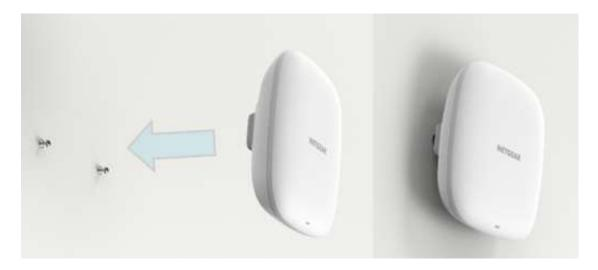
(Anchors size: Φ 8.00mm x L 25mm / Screws size: Φ 5.00mm x L 16mm)
