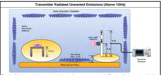
Electric field tests shall be performed in the frequency range of 1 GHz to 10th harmonic of highest fundamental frequency or 40 GHz using a calibrated horn antenna.
