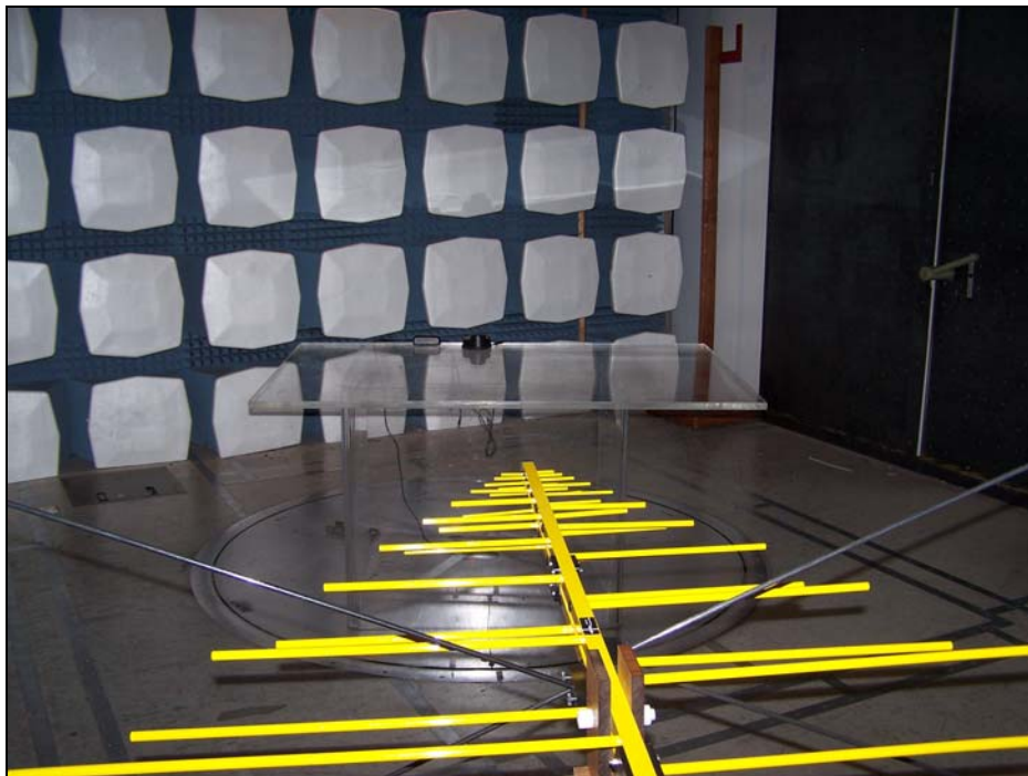
Photograph 2. Radiated Emission Test Setup (30 MHz to 1 GHz)
