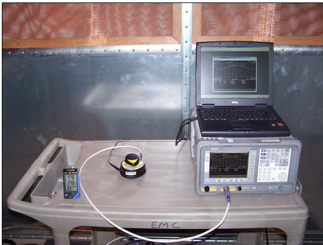
Photograph 4. 6 dB Bandwidth Test Setup
