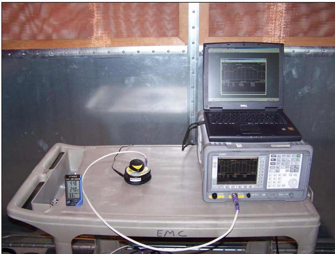
Photograph 7. Peak Power Spectral Density Test Setup
