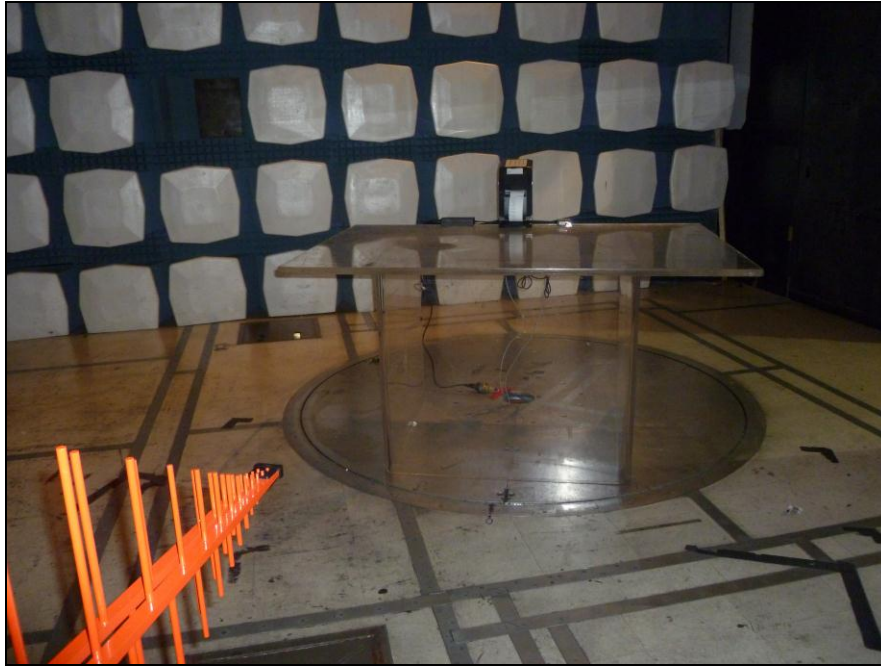
Photograph 3. Radiated Emission, Test Setup, Below 1 GHz
