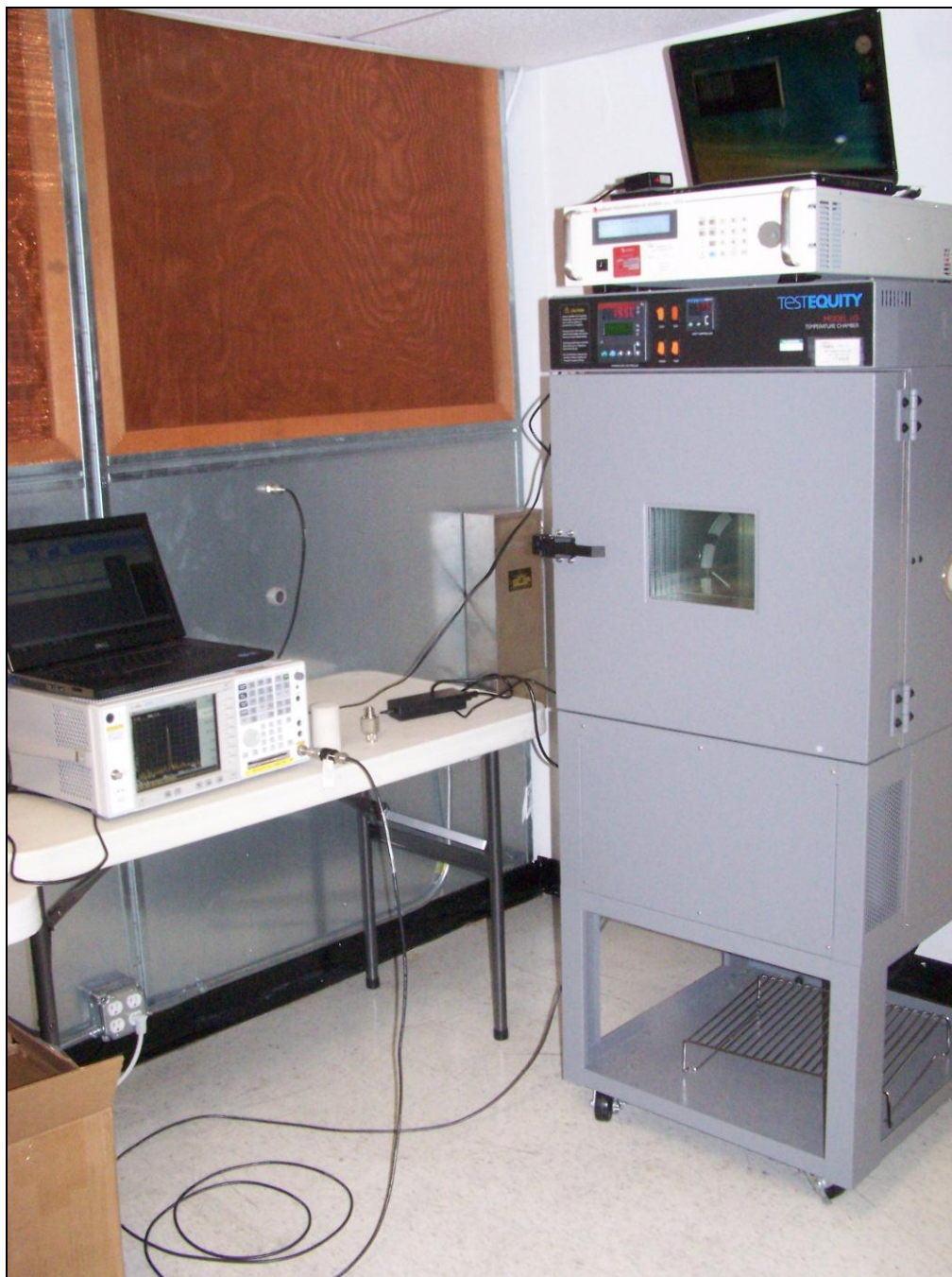
Photograph 9. Frequency Stability, Test Setup
