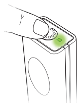
Tap the top of the microphone to check that the sound is heard in the hearing instruments
