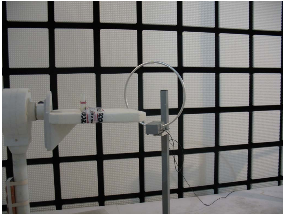
Photo 7: Test setup for near field measurements
