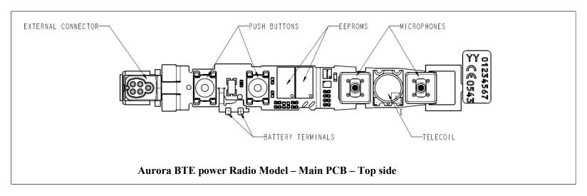
The most important part of the radio model is the Engine Module mounted on the main flex PCB, which connects it to both the EEPROM memory and all external connections: On the top side, these are the microphones, the battery terminals, the external connector and the push button.
