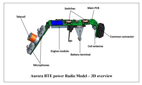
The radio model is implemented in an engine module mounted on the main PCB with connections to the antennas, the microphones, the speaker and the battery terminals. The radio model can be seen in 3D overview to the left:
