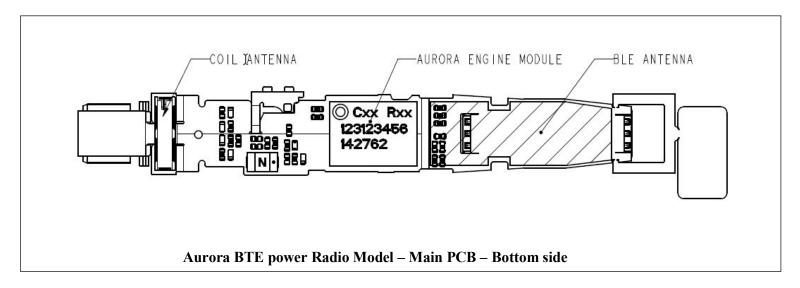
The most important parts inside the Engine module are a Digital-Signal-Processor (DSP), a radio Front-End (FE) chip for the 3.84 MHz radio part and an RF chip for the Bluetooth radio part – all mounted on a small rigid PCB again mounted on the main flex PCB. The Aurora BTE power radio model also includes all voltage regulators and buffered data programming inputs on-board. The DSP is the main processor controlling the functionality of both radios in the Aurora BTE power radio model.
