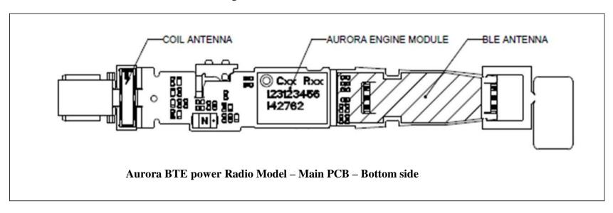
The most important parts inside the Engine module are a Digital-Signal-Processor (DSP), a radio Front-End (FE) chip for the 3.84 MHz radio part and an RF chip for the Bluetooth radio part – all mounted on a small rigid PCB again mounted on the main flex PCB. The Aurora BTE power radio model also includes all voltage regulators and buffered data programming inputs on board. The DSP is the main processor controlling the functionality of both radios in the radio model.
