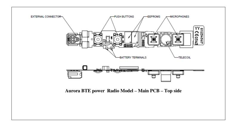
The 3.84 MHz radio is a low power, short range, inductive radio transceiver working at a single channel at 3.84 MHz using MSK modulation with 320 kbit/s data rate and connected to a small coil antenna.
