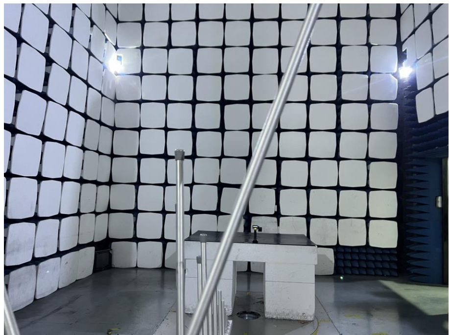
Radiation Emission Test Setup (30MHz to 1GHz)
