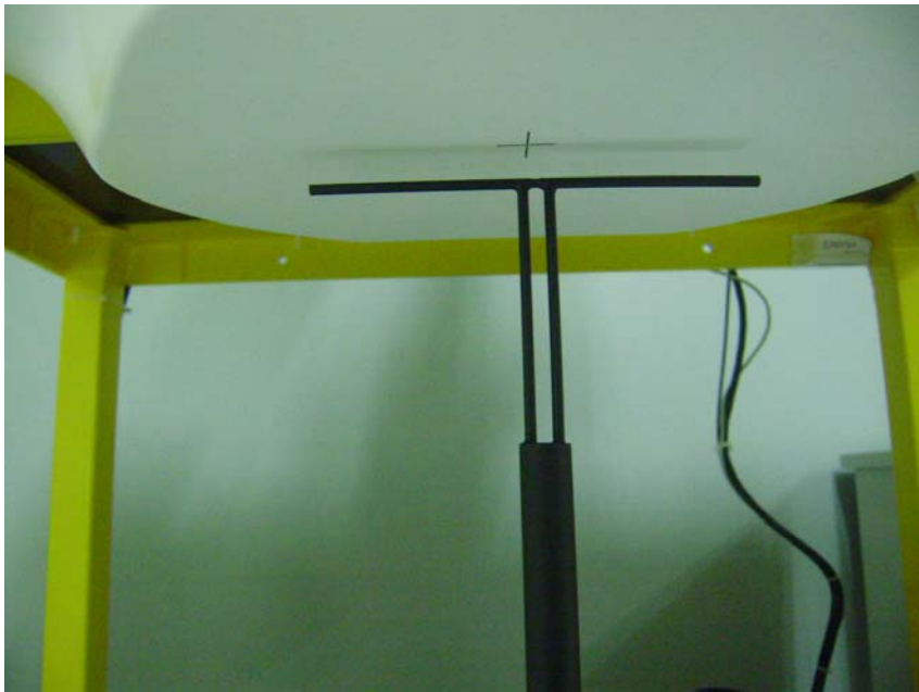
Setup Photo of Dipole Antenna
