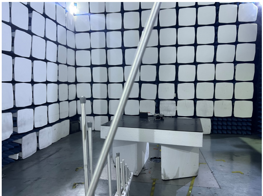
Radiation Emission Test Setup (30MHz to 1GHz)
