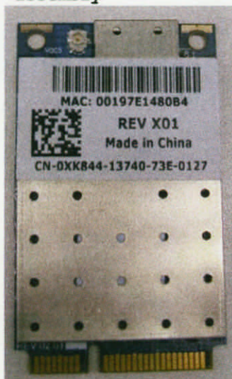
WiQuest Module PCB assembly
