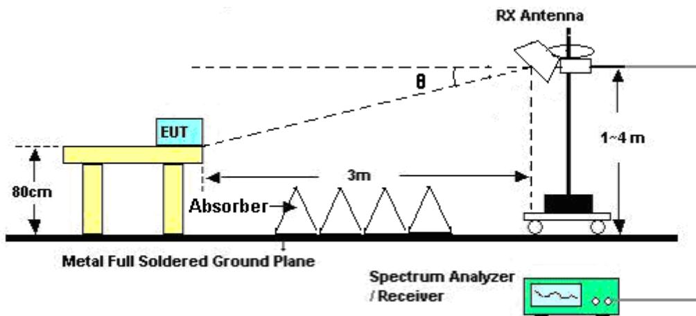
Note: The Horn Antenna maintaining bore sight alignment.
