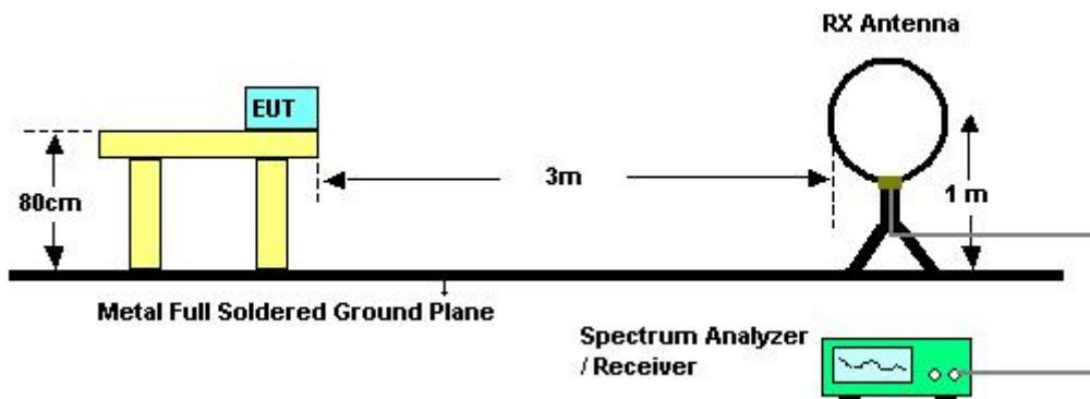
**For radiated emissions from 30MHz~1GHz**
