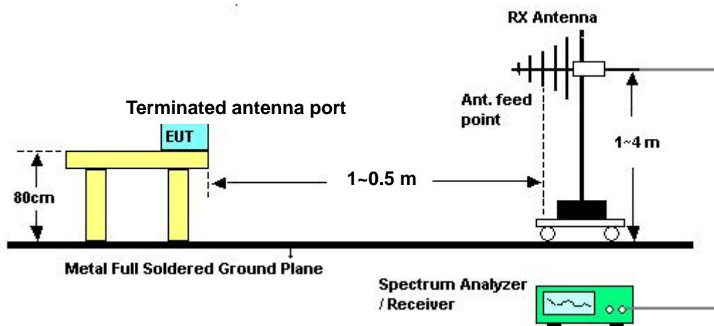
**For conducted emissions above 960MHz (Conducted antenna port measurement)**
