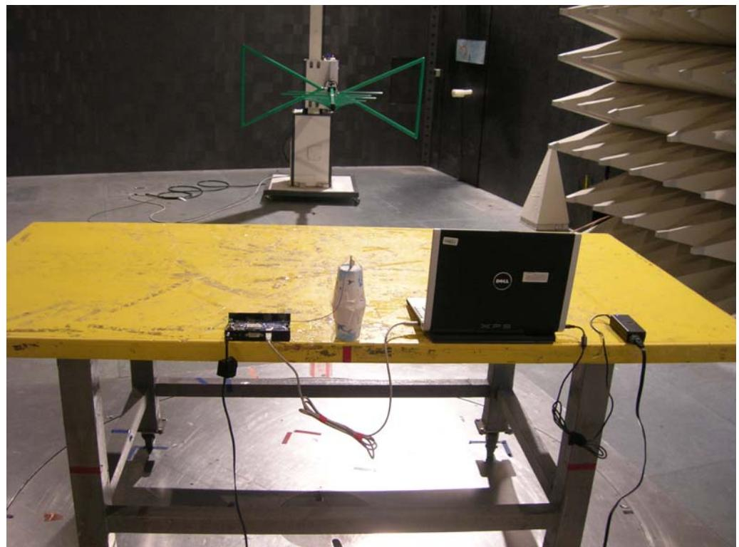
For radiated emissions from 3GHz to 5GHz
