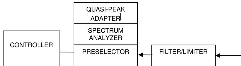
**FIGURE 2: Radiated Emissions Test Setup**
