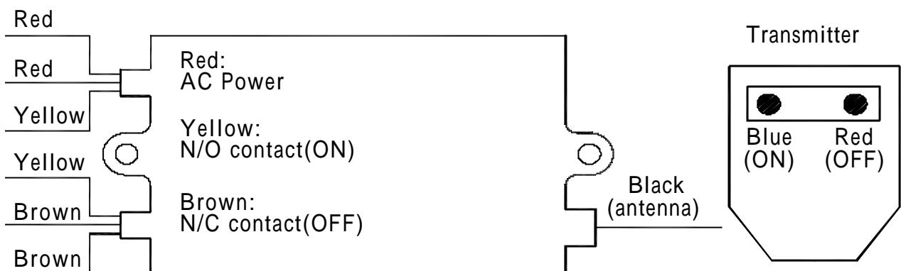
Motor Starter And Remote Controller Diagram :
