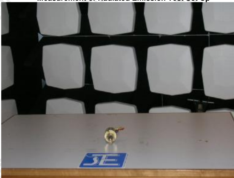
Measurement of Radiated Emission Test Set Up
