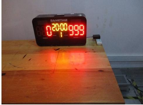
1.2 Radiated Spurious Emissions(30MHz~1GHz) Test Setup
