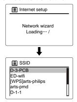
Rotate the DOWN/UP knob to select your Internet network (SSID) and then press DOWN/UP knob.
