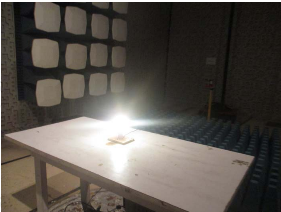
TEST SETUP OF RADIATED EMISSION (above 1GHz)
