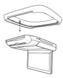
The trim ring is used to make the monitor sit flush against the ceiling contour. Ask ALPINE dealer for detail.
