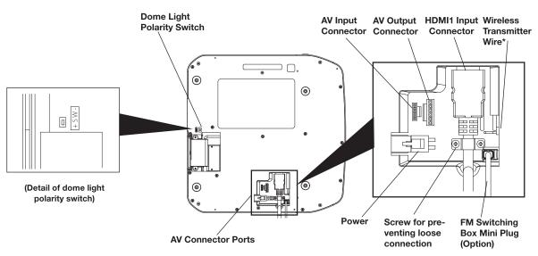
(Detail of AV connector ports)
