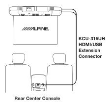
Route the connector to the center console through B Pillar from inside of headliner.
