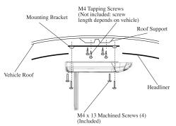
Install trim ring before attaching the overhead monitor to the metal installation bracket.
