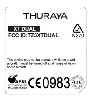
The FCC ID label will be affixed to the battery compartment of the Phone. The FCC ID shown in the FCC ID label page will be readily visible at the time of purchase because the phone will be marketed without the battery installed.
