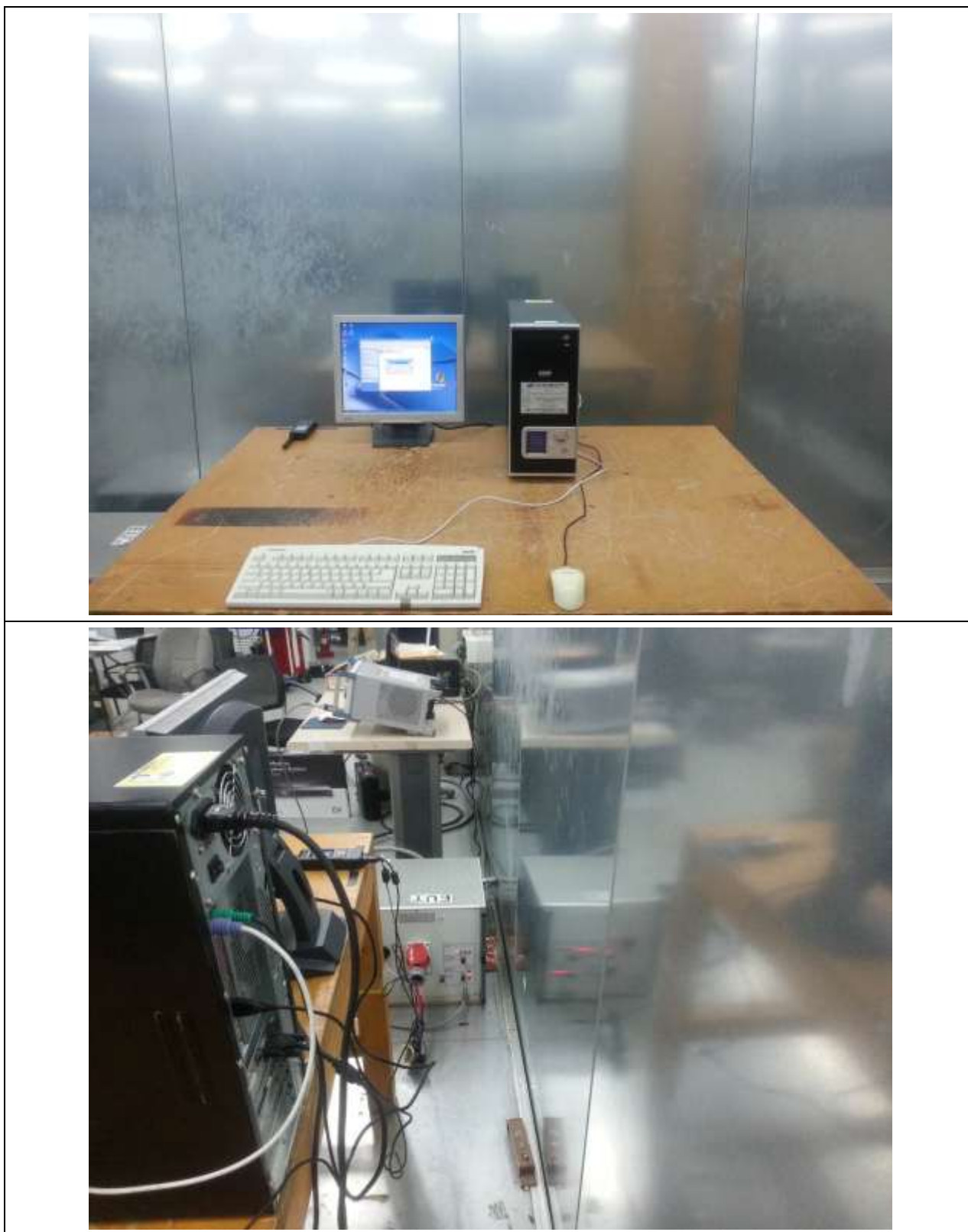
Figure 1. Test Setup for Conducted Emissions
