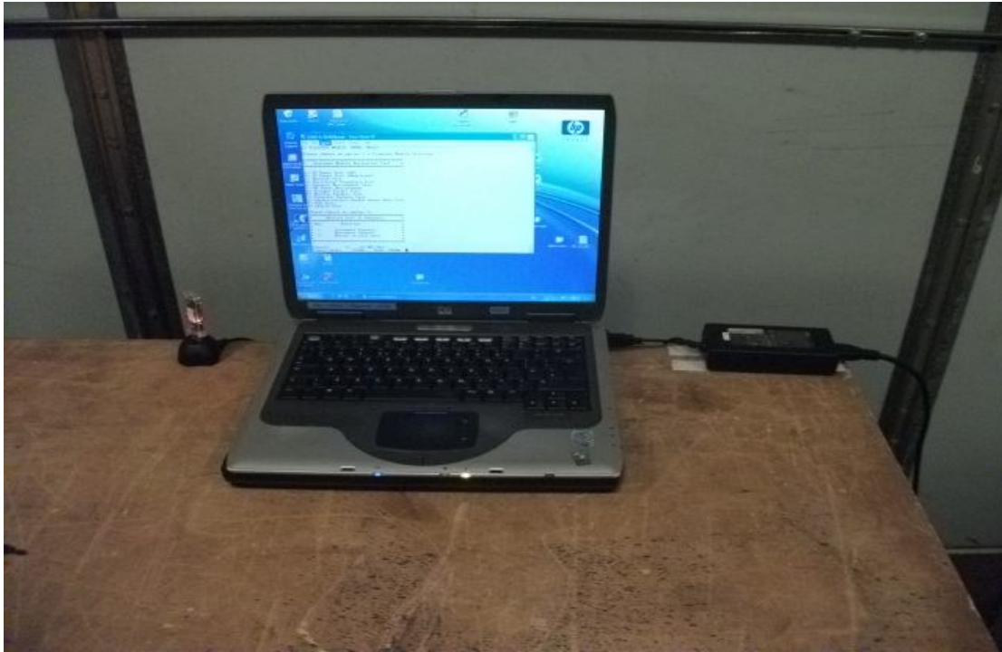
Photograph of the EUT as viewed from screened room (conducted emissions)
