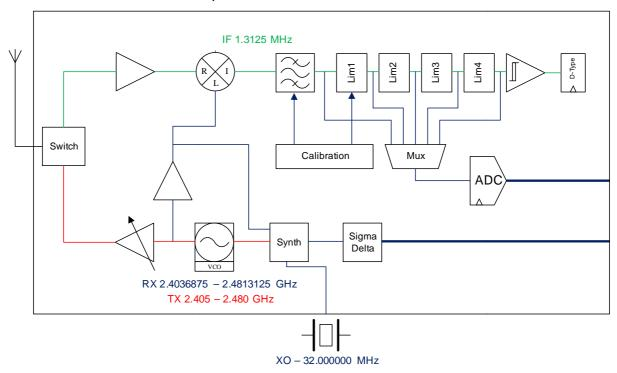
**Figure 1: Radio Architecture**
