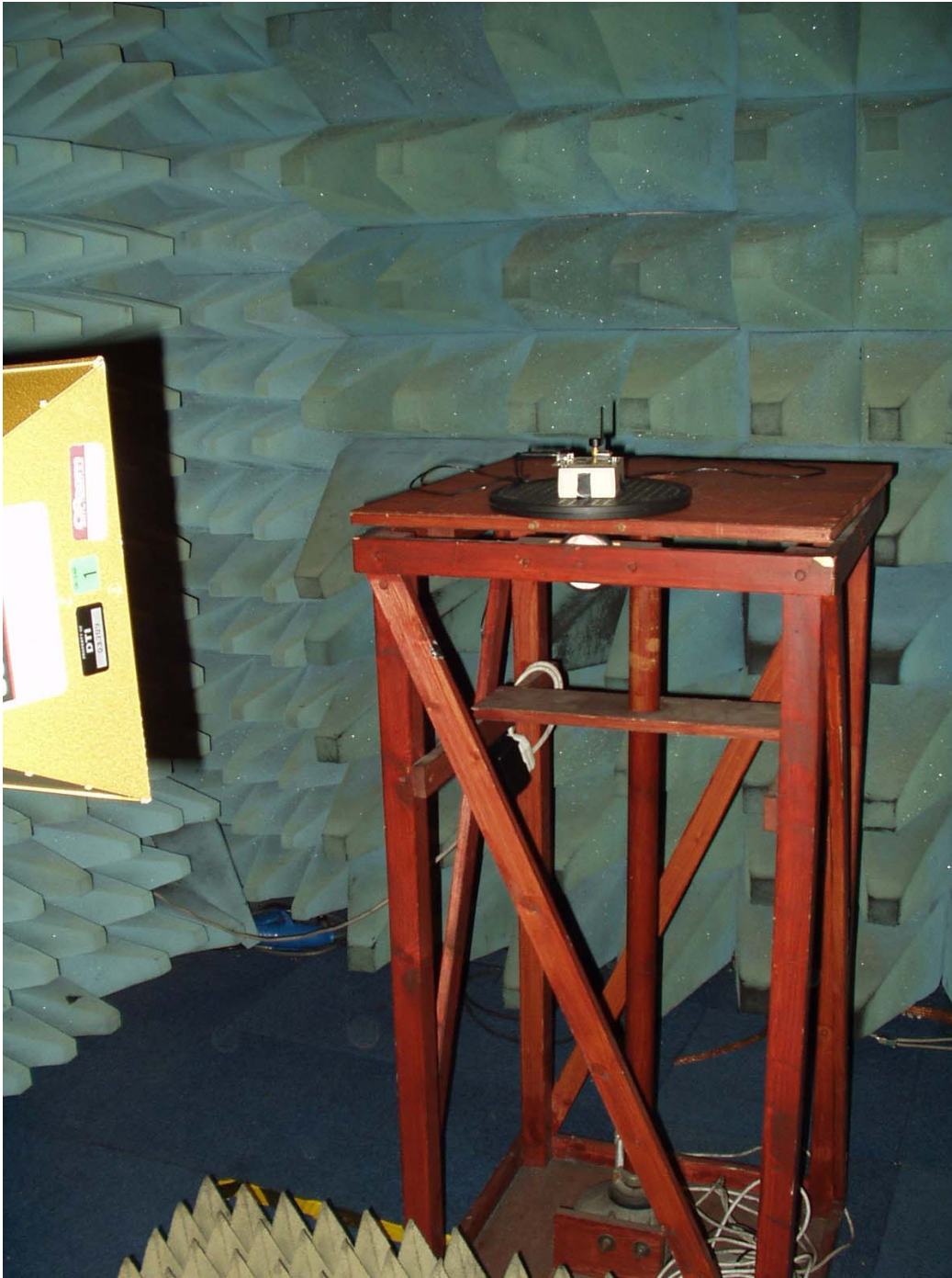
Photograph of the EUT as viewed from in front of the antenna, site M. EUT is mounted on a test jig on a turntable with test jig power adaptor to rear.
