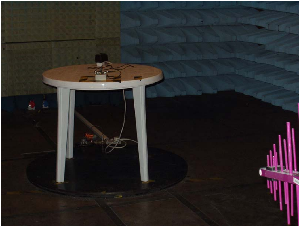
Photograph of the EUT as viewed from in front of the antenna, site M. EUT is mounted on a test jig on a turntable with test jig power adaptor to rear.
