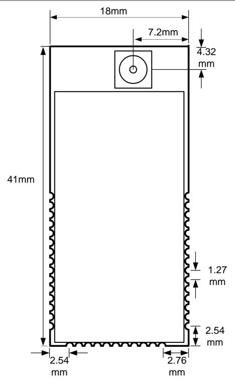
Thickness: 3.5mm over can, 10.8mm at SMA connector.
