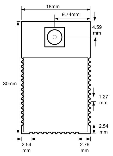
Thickness: 3.5mm over can, 10.8mm at SMA connector
