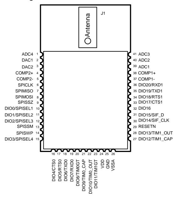
Figure 1: Pin Configuration (top view)
