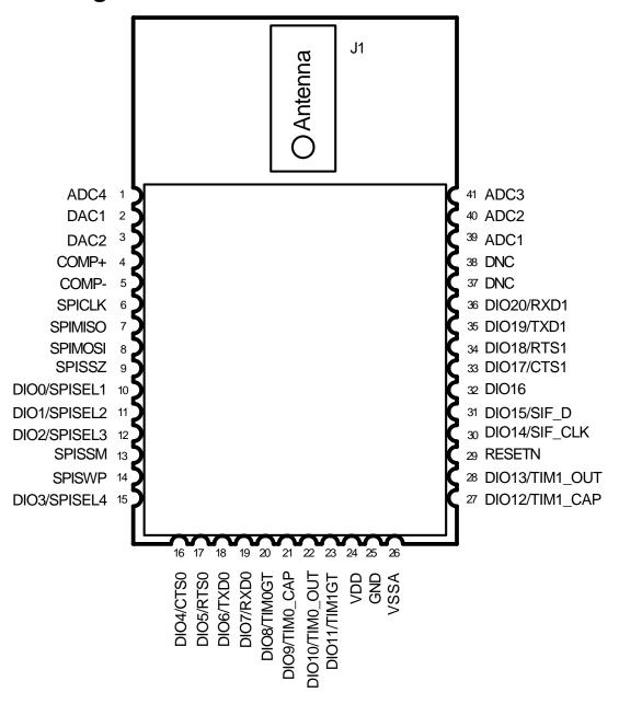
Figure 1: Pin Configuration (top view)
