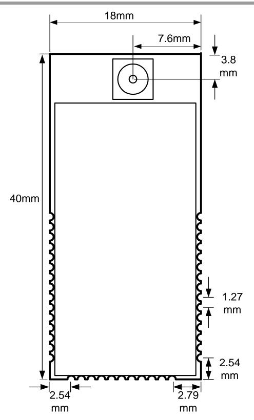
Thickness: 3mm, 10.6mm at SMA connector
