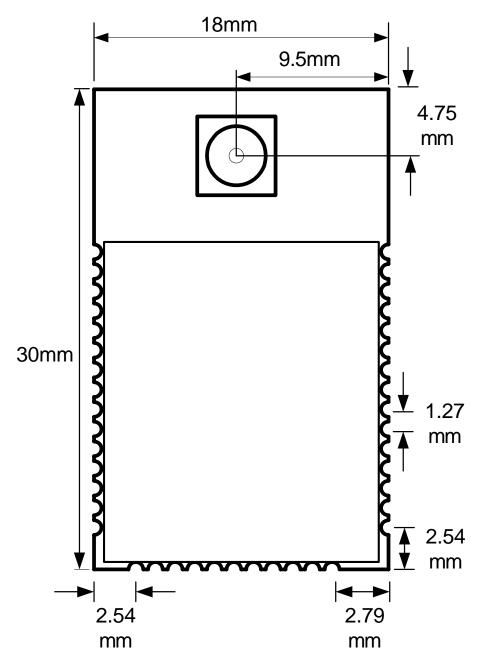
Thickness: 3mm over can, 10.6mm at SMA connector
