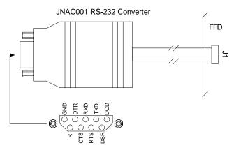
Figure 5-1: JNAC001 RS-232 Converter Connection
