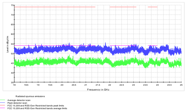
Figure 8.7-21: Radiated spurious emissions above 18 GHz for GFSK modulation mid channel
