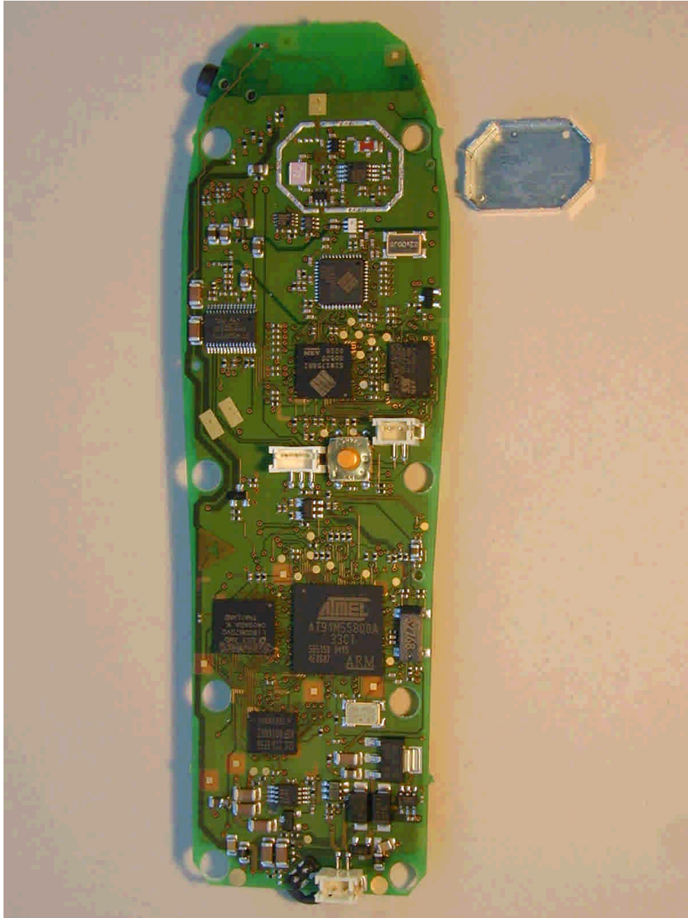
52105_18.jpg EXPLORER Bluetooth handset, PCB, top view, shielding removed
