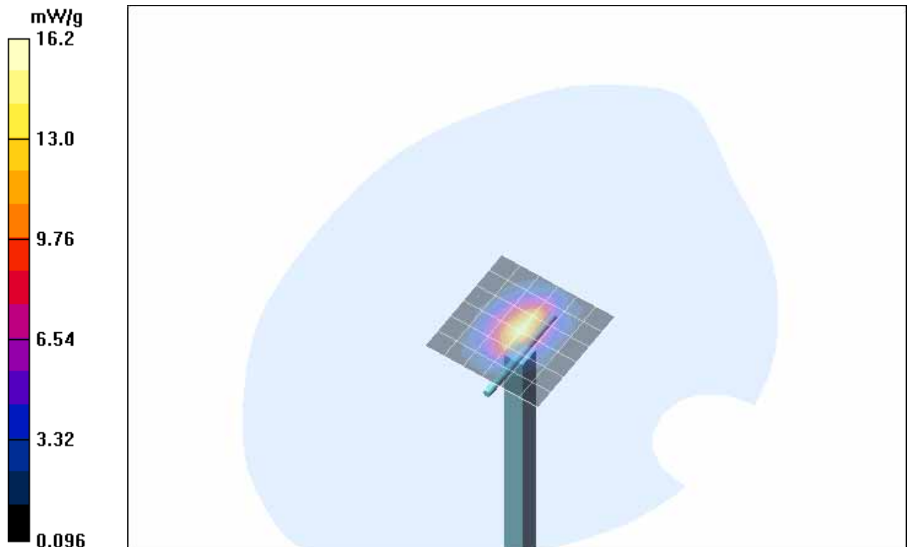
Fig. 9: Validation measurement 2450 MHz body (July 06, 2006), coarse grid. Ambient Temperature: 22.5° C, Liquid Temperature: 21.4° C.
