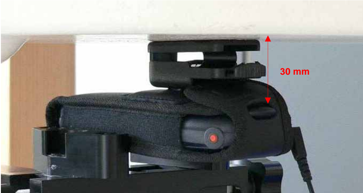
Fig. 18: Picture of the device tested with leather case, rotation clip and headset.
