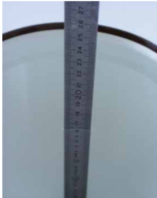
Fig. 18: Liquid depth for 2450 MHz Head measurements.
