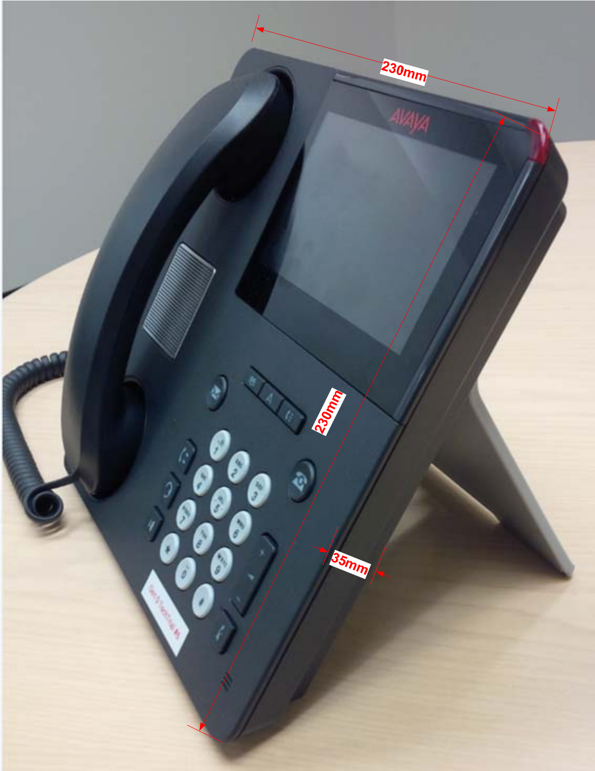
Figure 1: 9641GS Perspective view with Dimensions 230mm x 230mm x 35mm
