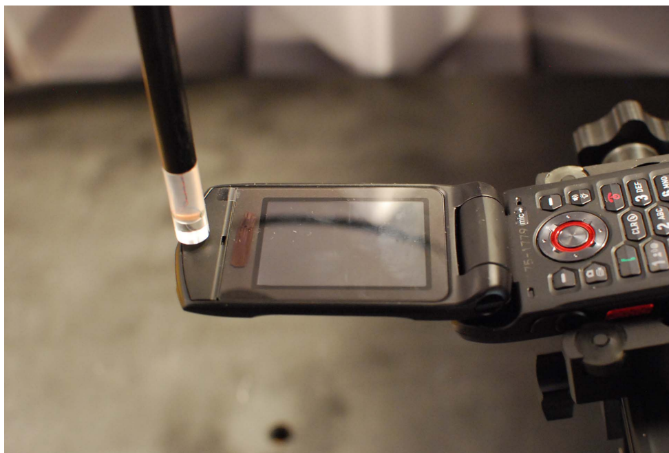
Figure 13-2 Test Setup for Wireless Device
