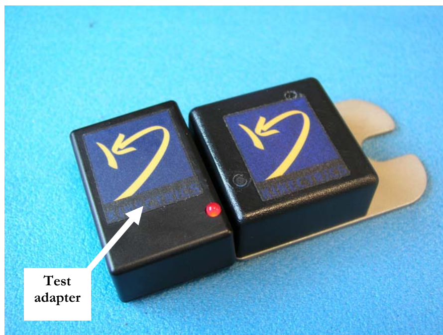
Figure 3 – Test Adapter connected to the RST. Care should be taken in aligning the pins appropriately. The test adapter will be centred and the red LED will illuminate when installed properly.
