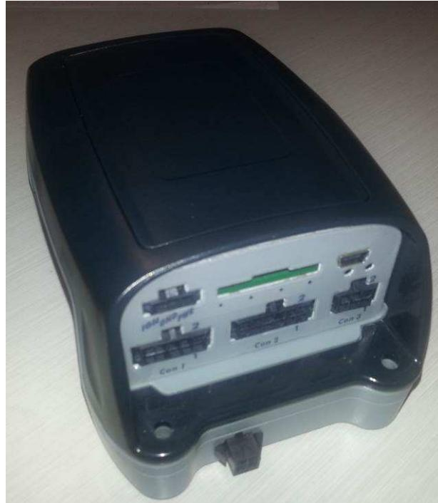
To accommodate the PLC interface the device has alternate plastics which are slightly taller than the Vector 301-IW.
