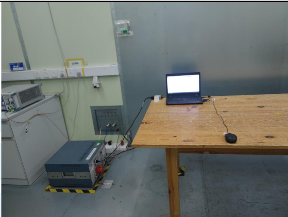
Conducted Emission Test Setup
