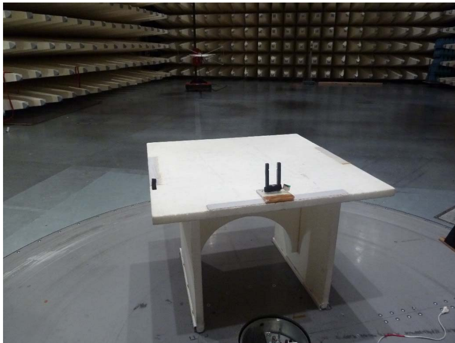
Photo 7: EUT at the semi-anechoic chamber
