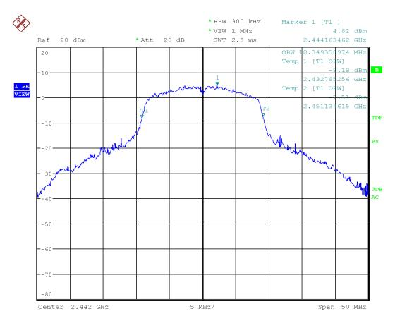
Figure 22: Chart of occupied bandwidth test on middle channel, IEEE 802.11 n (HT20)
