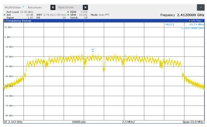
Figure 39: Chart of power spectral density on lowest channel, IEEE 802.11 n (HT20)
