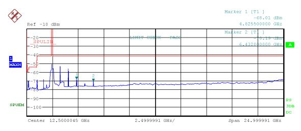
Figure 58: Chart of emissions test from 9 kHz to 25 GHz on lowest channel, RMS-detector, IEEE 802.11 g
