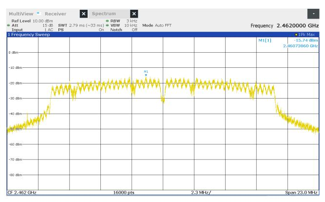
Figure 38: Chart of power spectral density on highest channel, IEEE 802.11 g
