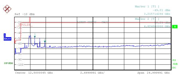
Figure 51: Chart of emissions test from 9 kHz to 25 GHz on lowest channel, PK-detector, IEEE 802.11 b
