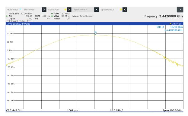
Figure 28: Chart of conducted output power on middle channel, IEEE 802.11 g
