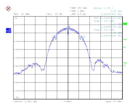
Figure 16: Chart of occupied bandwidth test on middle channel, IEEE 802.11 b
