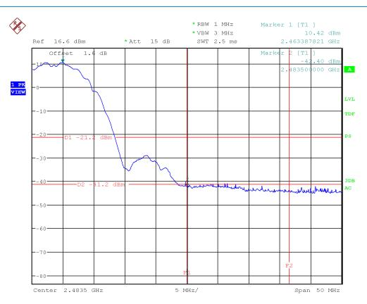
Figure 43: Chart of band-edge measurement on highest channel (PK), IEEE 802.11 b
