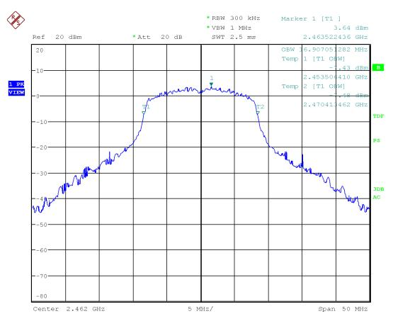
Figure 20: Chart of occupied bandwidth test on highest channel, IEEE 802.11 g
