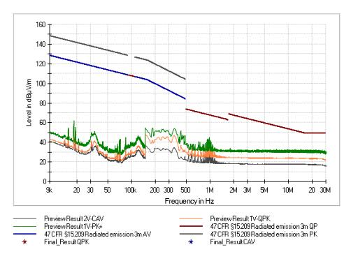
Figure 69: Chart of emissions test below 30 MHz on highest channel, EUT position X, antenna parallel to the EUT
