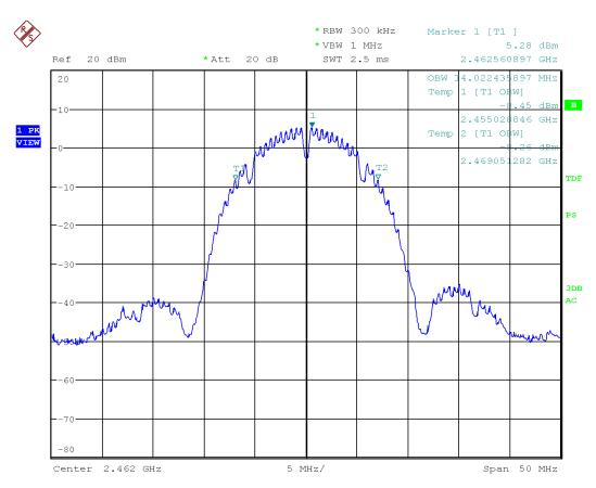
Figure 17: Chart of occupied bandwidth test on highest channel, IEEE 802.11 b
