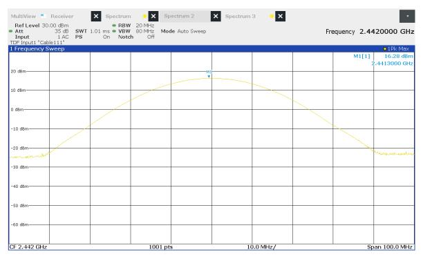
Figure 25: Chart of conducted output power on middle channel, IEEE 802.11 b
