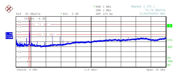
Figure 73: Chart of emissions test from 1 GHz to 17 GHz on middle channel, EUT position Z, antenna polarization horizontal
