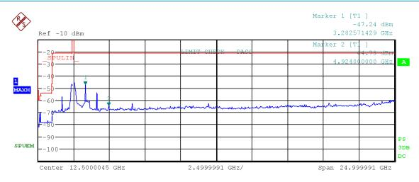
Figure 67: Chart of emissions test from 9 kHz to 25 GHz on highest channel, PK-detector, IEEE 802.11 n (HT20)
