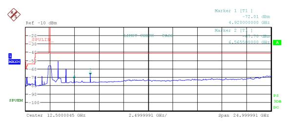
Figure 62: Chart of emissions test from 9 kHz to 25 GHz on highest channel, RMS-detector, IEEE 802.11 g
