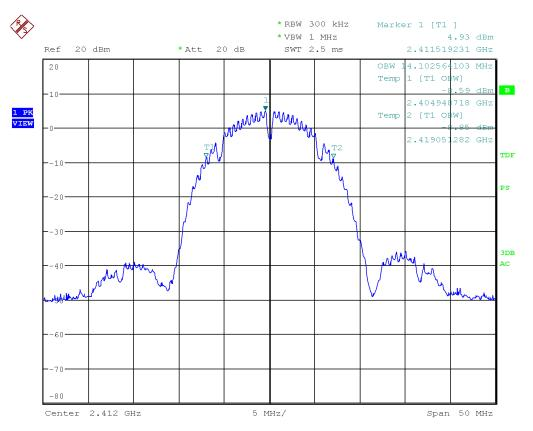
Figure 15: Chart of occupied bandwidth test on lowest channel, IEEE 802.11 b
