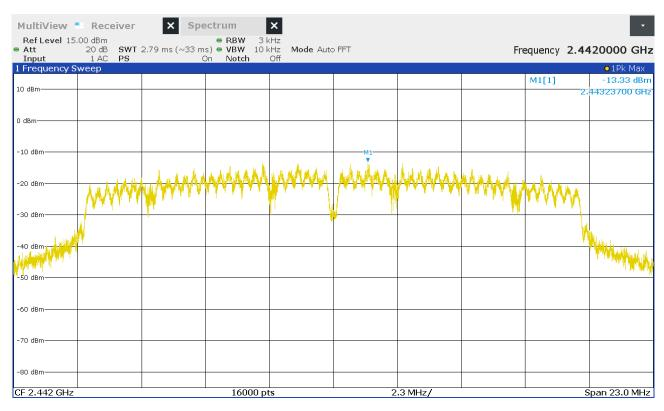
Figure 40: Chart of power spectral density on middle channel, IEEE 802.11 n (HT20)
