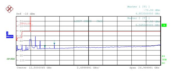
Figure 68: Chart of emissions test from 9 kHz to 25 GHz on highest channel, RMS-detector, IEEE 802.11 n (HT20)
