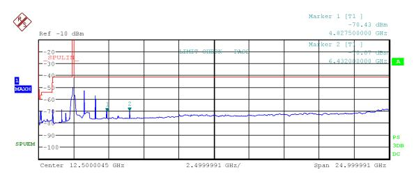
Figure 64: Chart of emissions test from 9 kHz to 25 GHz on lowest channel, RMS-detector, IEEE 802.11 n (HT20)
