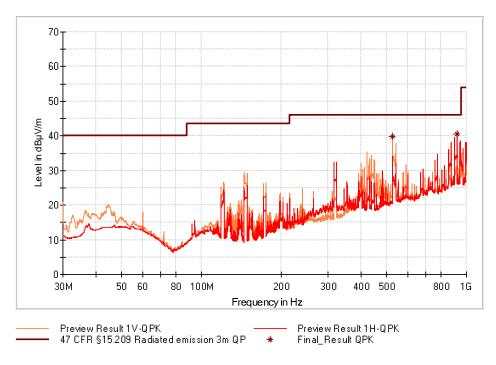
Figure 70: Chart of emissions test from 30 MHz to 1 GHz on lowest channel, EUT position Y
