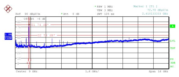
Figure 71: Chart of emissions test from 1 GHz to 17 GHz on lowest channel, EUT position Z, antenna polarization horizontal
