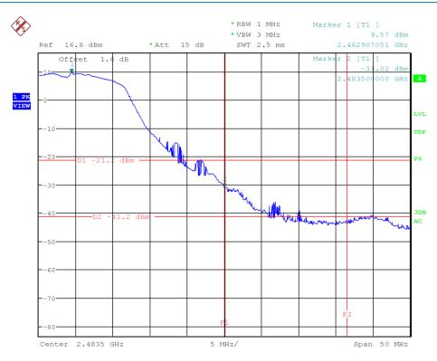
Figure 49: Chart of band-edge measurement on highest channel (PK), IEEE 802.11 n (HT20)
