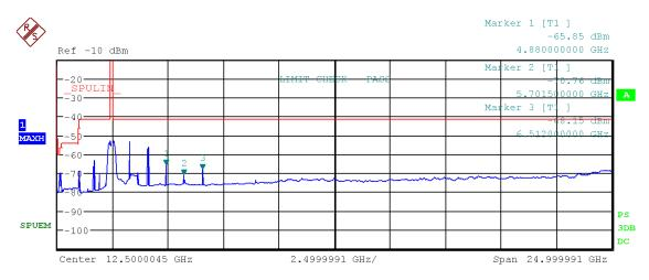
Figure 60: Chart of emissions test from 9 kHz to 25 GHz on middle channel, RMS-detector, IEEE 802.11 g
