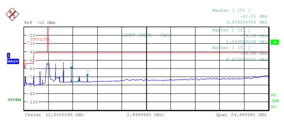
Figure 52: Chart of emissions test from 9 kHz to 25 GHz on lowest channel, RMS-detector, IEEE 802.11 b
