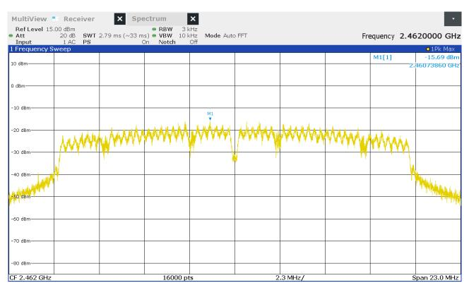
Figure 41: Chart of power spectral density on highest channel, IEEE 802.11 n (HT20)
