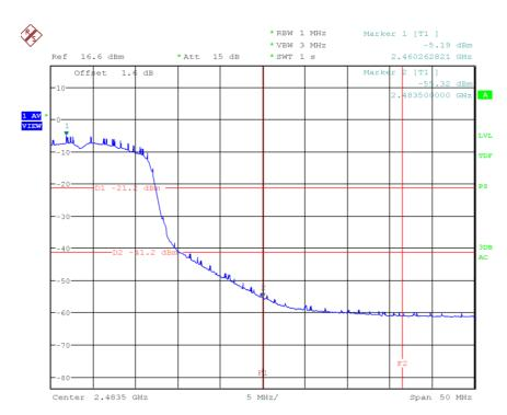
Figure 47: Chart of band-edge measurement on highest channel (AV), IEEE 802.11 g
