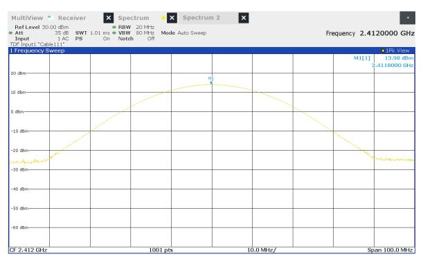
Figure 24: Chart of conducted output power on lowest channel, IEEE 802.11 b
