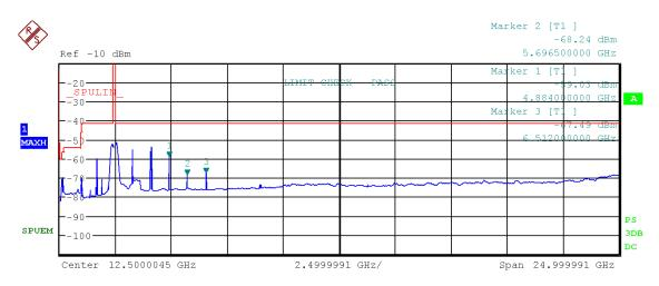
Figure 54: Chart of emissions test from 9 kHz to 25 GHz on middle channel, RMS-detector, IEEE 802.11 b
