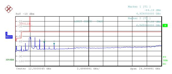
Figure 56: Chart of emissions test from 9 kHz to 25 GHz on highest channel, RMS-detector, IEEE 802.11 b
