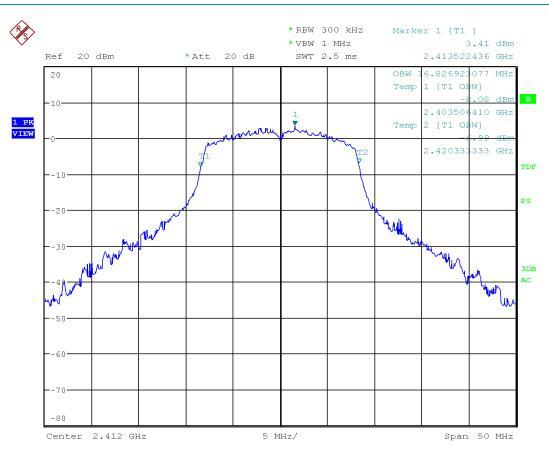
Figure 18: Chart of occupied bandwidth test on lowest channel, IEEE 802.11 g
