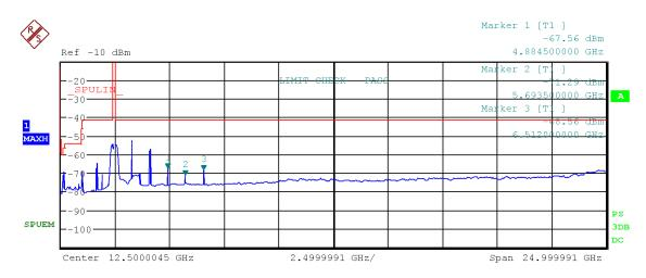
Figure 66: Chart of emissions test from 9 kHz to 25 GHz on middle channel, RMS-detector, IEEE 802.11 n (HT20)
