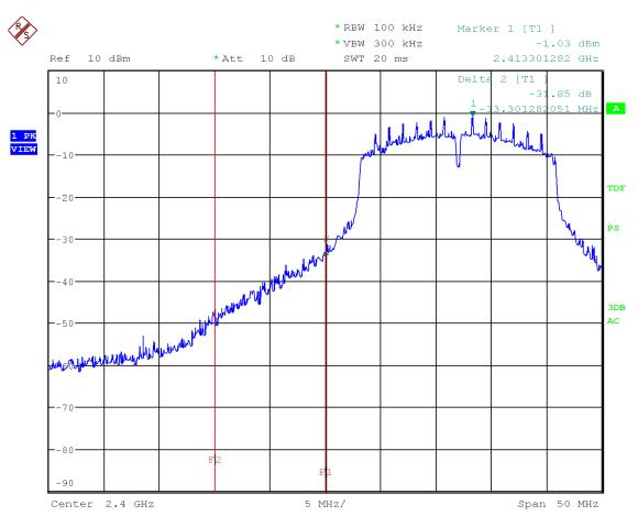
Figure 48: Chart of band-edge measurement on lowest channel, IEEE 802.11 n (HT20)
