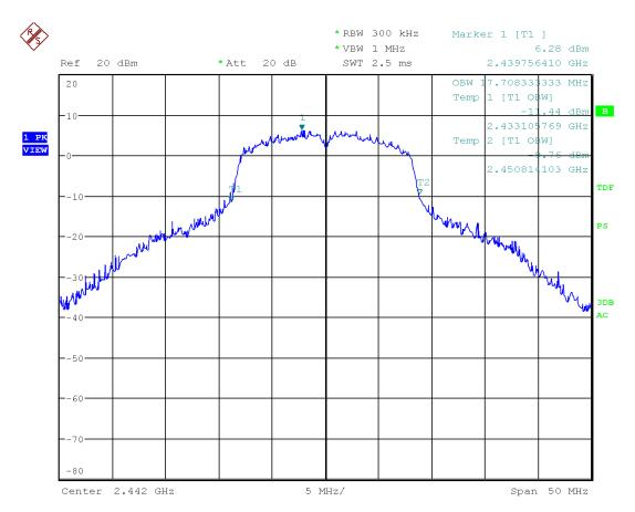
Figure 19: Chart of occupied bandwidth test on middle channel, IEEE 802.11 g
