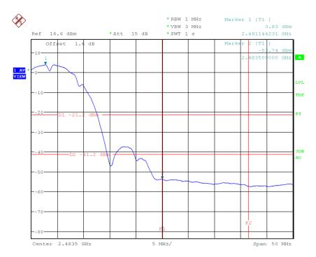
Figure 44: Chart of band-edge measurement on highest channel (AV), IEEE 802.11 b
