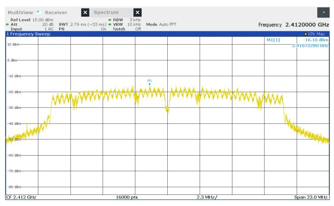
Figure 36: Chart of power spectral density on lowest channel, IEEE 802.11 g
