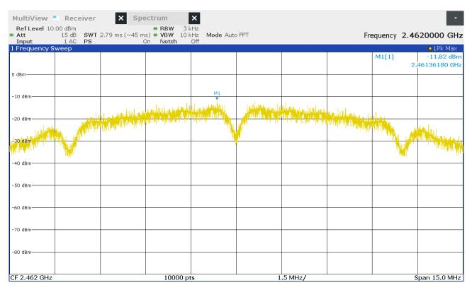
Figure 35: Chart of power spectral density on highest channel, IEEE 802.11 b
