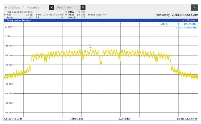
Figure 37: Chart of power spectral density on middle channel, IEEE 802.11 g
