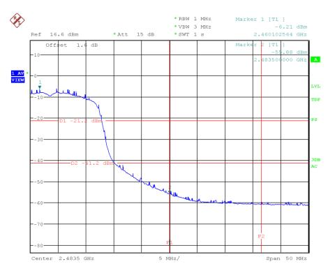
Figure 50: Chart of band-edge measurement on highest channel (AV), IEEE 802.11 n (HT20)
