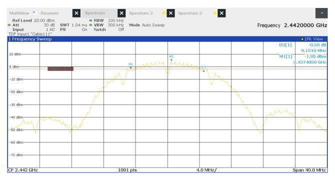
Figure 7: Chart of 6 dB bandwidth test on middle channel, IEEE 802.11 b
