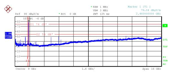
Figure 75: Chart of emissions test from 1 GHz to 17 GHz on highest channel, EUT position Z, antenna polarization horizontal
