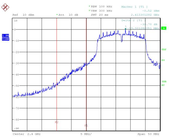
Figure 45: Chart of band-edge measurement on lowest channel, IEEE 802.11 g
