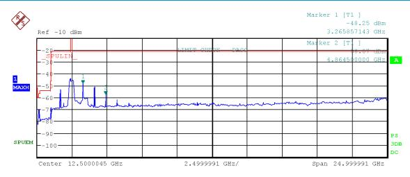
Figure 65: Chart of emissions test from 9 kHz to 25 GHz on middle channel, PK-detector, IEEE 802.11 n (HT20)
