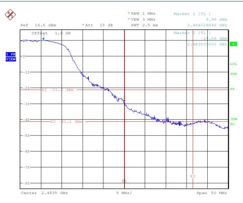
Figure 46: Chart of band-edge measurement on highest channel (PK), IEEE 802.11 g
