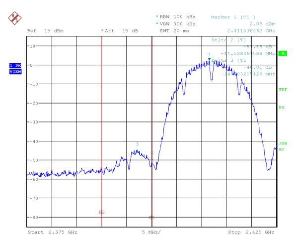
Figure 42: Chart of band-edge measurement on lowest channel, IEEE 802.11 b
