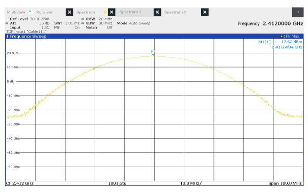
Figure 27: Chart of conducted output power on lowest channel, IEEE 802.11 g
