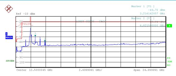
Figure 63: Chart of emissions test from 9 kHz to 25 GHz on lowest channel, PK-detector, IEEE 802.11 n (HT20)
