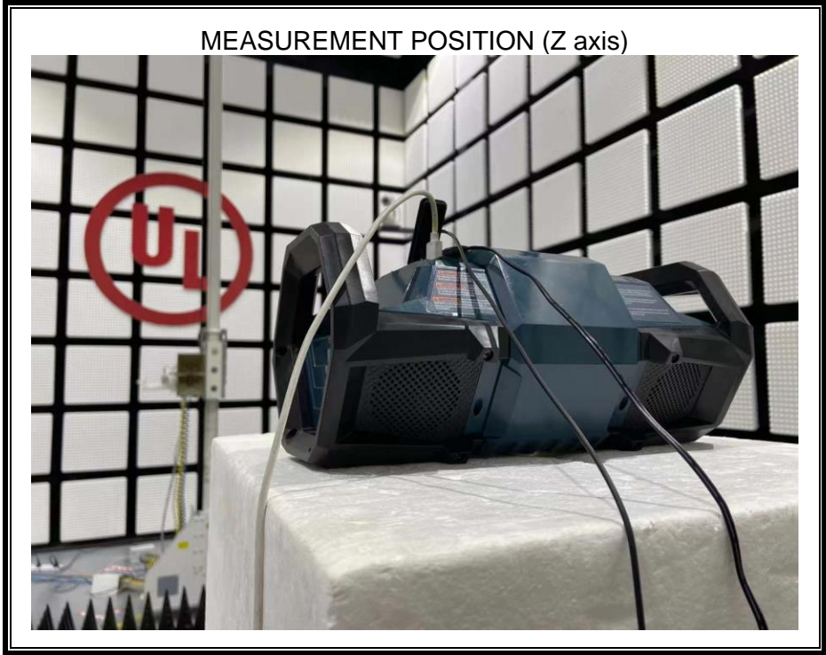
RADIATED RF MEASUREMENT SETUP (30MHz~1GHz)
