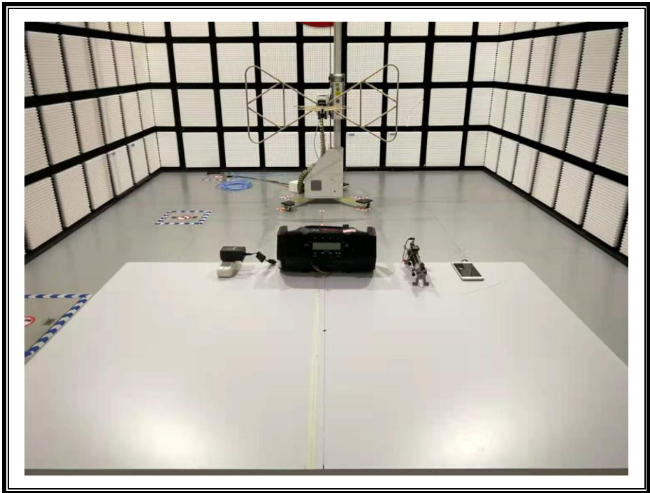
RADIATED RF MEASUREMENT SETUP (30MHz~1GHz)
