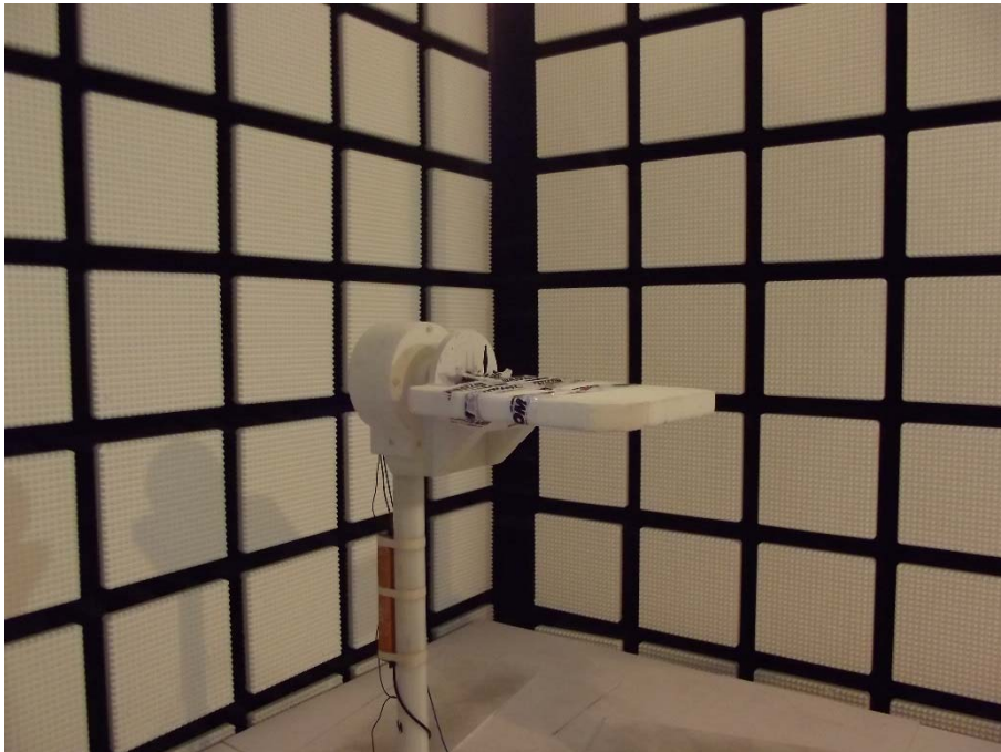
Photo 2: EUT at the anechoic chamber
