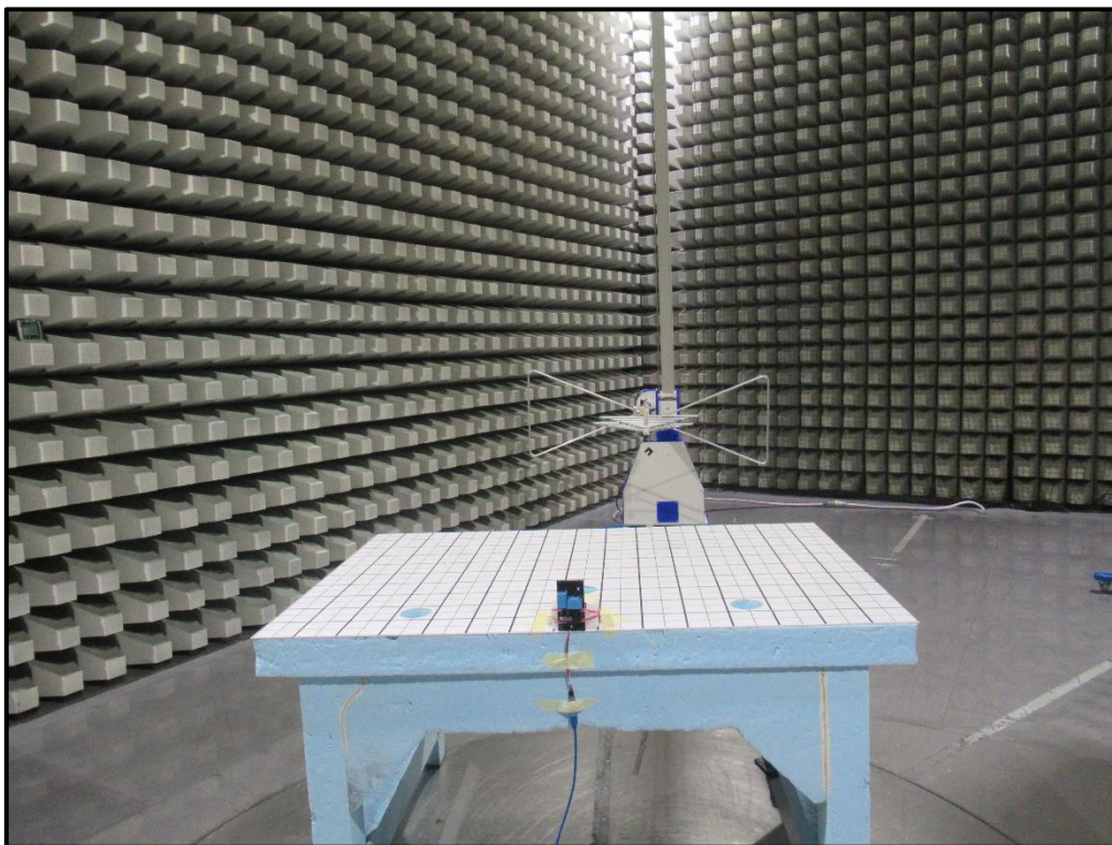
Photo 4: Radiated Test Setup-30 MHz to 1GHz
