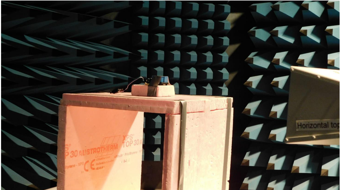
Picture 12: Setup for radiated measurement
