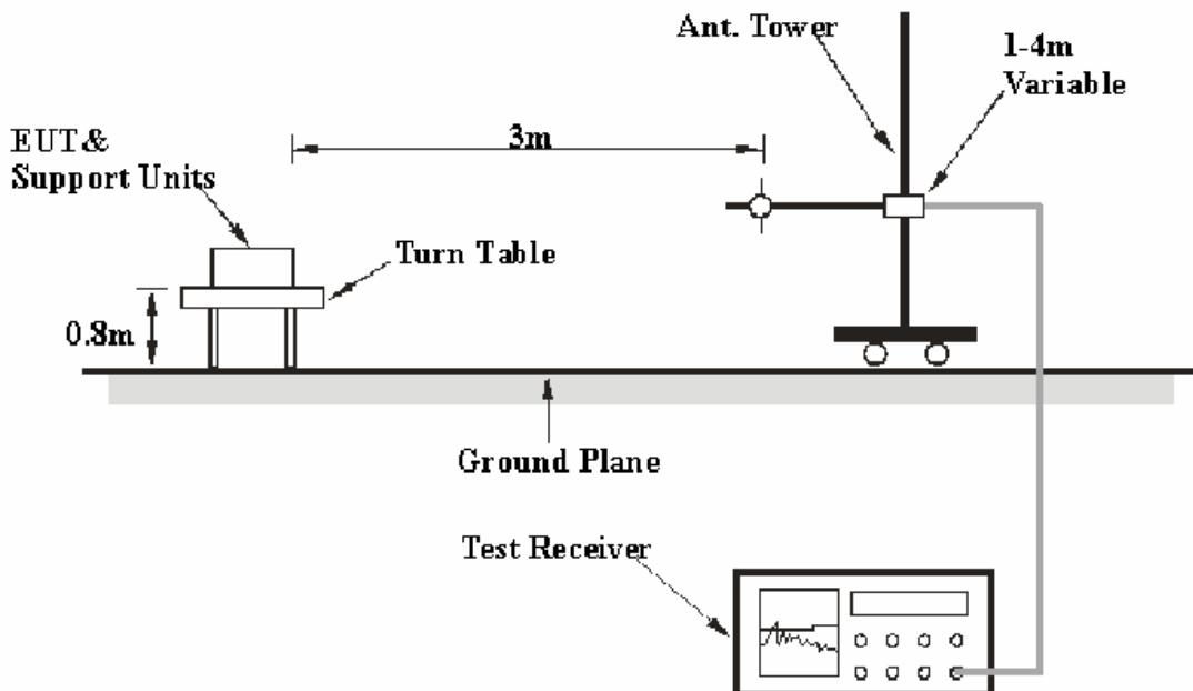
The deactivation test was performed in the 3 meters chamber B test site, using the setup accordance with the ANSI C63.4 - 2003. The specification used was the FCC 15.231(e) limits.
