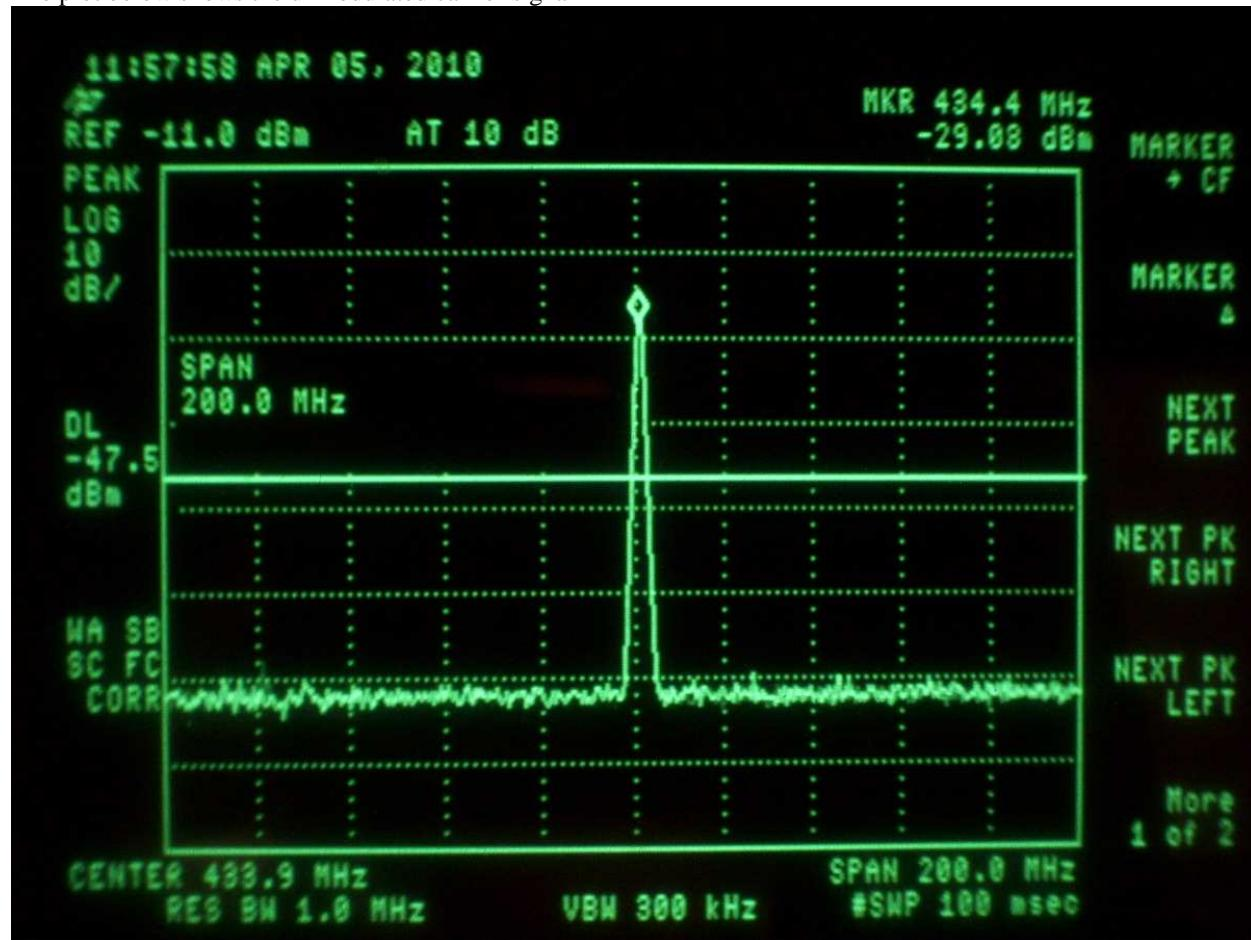
The plot below shows the modulated signal.
