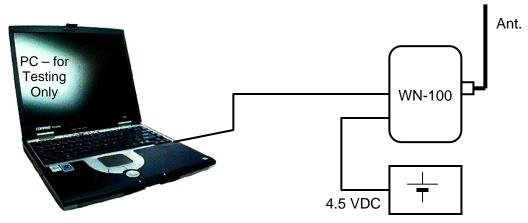
NOTE: The EUT is not a computer peripheral. The computer was used only to adjust the settings on the transceiver before the test and then disconnected.
