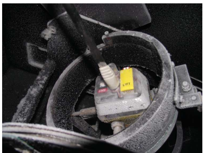
Figure 13.6 – View of the EUT upon completion of the low-duty cycle test at minimum temperature
