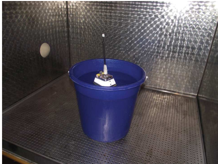
Figure 11.1 – View of the EUT in the temperature test chamber upon completion of the Thermal Shock Test
